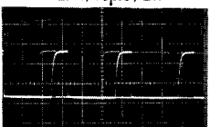
27. IC601 Pin 2 (E-PCB) Serial Clock Line 4.6V, 10 \mu s / Div
