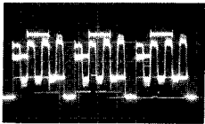
7. TP 18 (IC601 PIN 22) (E-PCB) 4.0V, 20 \mu s / Div
